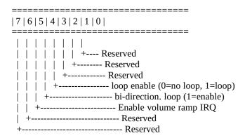
The bits that should be set by the application to get a particular type of volume ramp. The completed value should be supplied to UltraRampVolume and UltraRampLinearVolume. If volume interrupts are enabled, make sure that you have set up a volume interrupt handler (see UltraVolumeHandler). This can be used to create your own multipoint volume envelopes.
