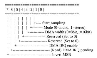
Bit 0 - If PC DMA controller is programmed, it will begin sampling as soon as this is enabled.
