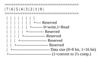
Note: The UltraSound DRAM location MUST be on a 32 byte boundary. UltraMemAlloc enforces this stipulation.
